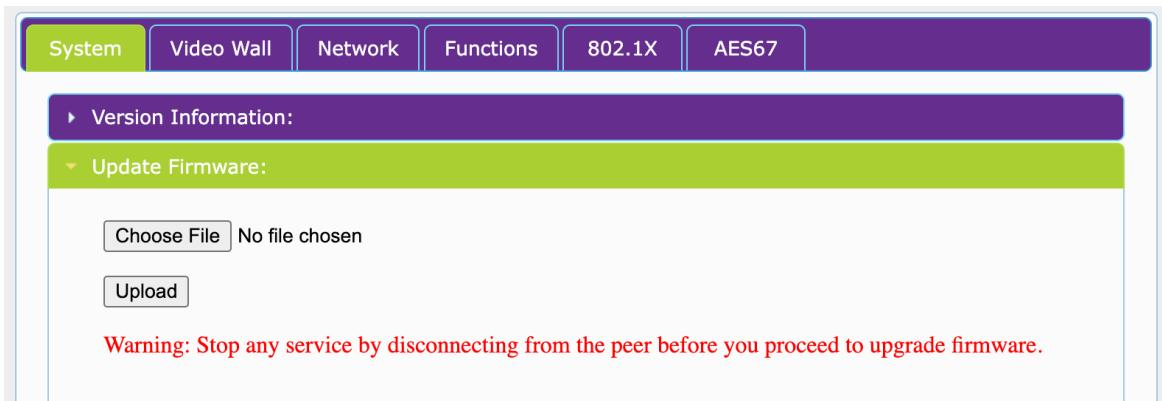
Choose the appropriate firmware update file that you have obtained from ZeeVee and press the Upload button. Note this process will force the encoder or decoder unit to reboot.
