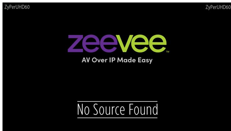
The default background can be changed from the ZyPer Management Platform GUI in the **Display Grid** page **Config** tab.
