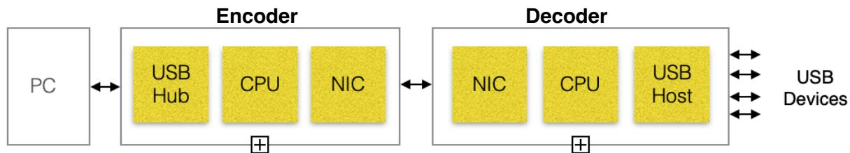
A ZyPerUHD60 System can support up to 6 decoders or “USB input devices” connected to a single encoder for USB Connections. The maximum number of supported USB endpoints connected back to an encoder over USB is 19.
