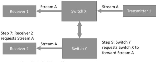
Step 10: Switch Y provides Receiver 2 Stream A
