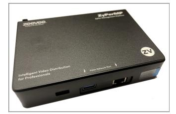
Installations will require a ZyPer Management Platform (ZMP). This device controls the operation and manages the connectivity between endpoints. The management platform is a hardened controller node that must reside on the same logical network as the ZyPer Encoders and Decoders. It runs a ZeeVee application as its sole function. The application presents an API to potential third party management platforms as well as hosting its own browser based management application.
