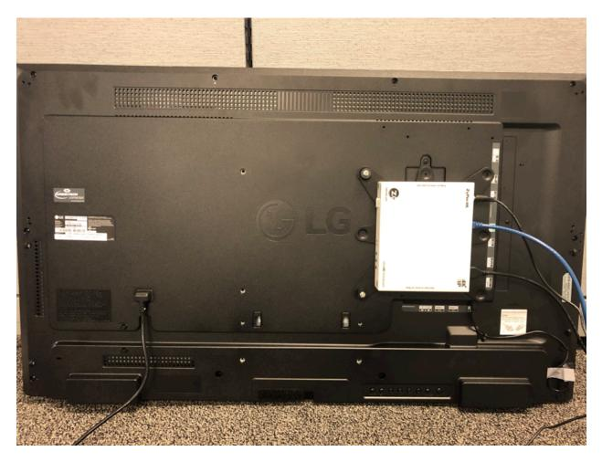
User should always ensure ZyPer4K units have free space above and below in these installations to provide needed air flow.
