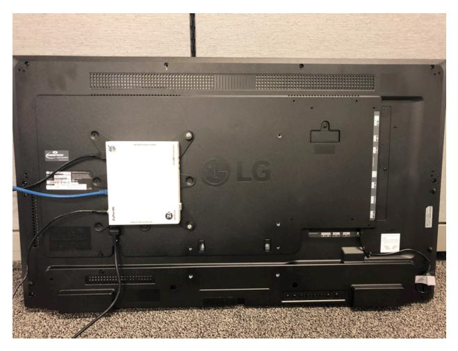
Example of ZyPer4K decoder mounted to right of 200 x 200mm VESA holes. Note the direction of ZyPer4K unit and cables. This mounting allows use of VESA holes for display mounting.
