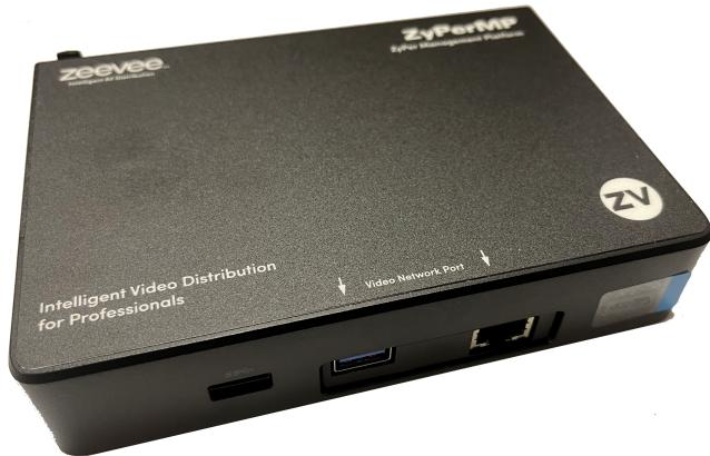
Installations will require a ZyPer Management Platform (ZyPerMP). This device controls the operation and manages the connectivity between endpoints. The management platform is a hardened controller node that must reside on the same logical network as the ZyPer4K Encoders and Decoders. It runs a ZeeVee application as its sole function. The application presents an API to potential third party management platforms as well as hosting its own management application.
