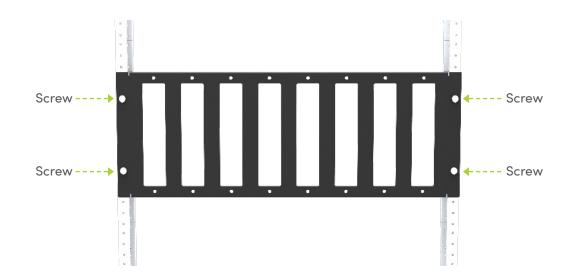
2. Install the ZyPer4K encoders/decoder in the carrier unit using the included 4-40 countersink screws. ZyPerUHD should use the screws already included with the ZyPerUHD units. Make sure that three screws are used to secure each device. Note that the ZyPer encoders/decoders can be positioned forward or backward within each carrier unit, depending upon your requirements.
