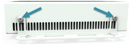
Sheet Metal Shelf or Equipment: #6 up to #10 thread-forming or thread-cutting machine screws. Pilot holes should be drilled using the equipment as an outline template. Should the removal of equipment periodically be required use thread-cutting screws. The recommended sequence of hardware would be; Flat Washer, ZyPer4K L-Bracket, Flat washer, Lock Washer (when using thread cutting screw), Screw or Bolt.
