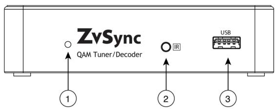
**1. LED Status Indicator** – Indicates state of unit. RED – Unit is powered-up and ACTIVATED
