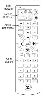
The ZvMX decoder is supplied with a partial learning remote control device. Buttons P1-P5 can be programmed to mimic the functions of a select set of buttons from another remote control unit.
