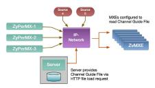
If the guide file is in "Additive" mode only the non-ZeeVee channels need to be specified in the guide file. The ZeeVee channels will send beacons that are learned by the ZvMXE and those channels will automatically be added to the guide. In the diagram shown Source4 and Source5 are streams supplied by non-ZeeVee equipment. Only stream information for Source 4. and Source 5 need to be specified in the guide file.
