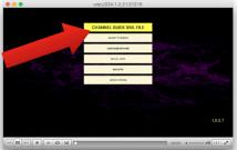
Navigate to, and click on the "CHANNEL GUIDE XML FILE" button
