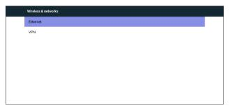
Ethernet MAC field is hard coded and cannot be changed.
