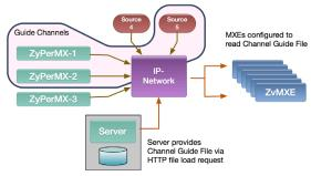
In the diagram shown, if the guide file is specified as exclusive, and the only entries in that guide file are for ZvPerMX-1, ZvPerMX-2, and Source 5, then any other channel will be ignored and not included in the guide. The only stream the user will be able to select are for the channels described in the quide file.
