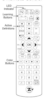
The ZvMXE+ decoder is supplied with a partial learning remote control device. Buttons P1-P5 can be programmed to mimic the functions of a select set of buttons from another remote control unit.
