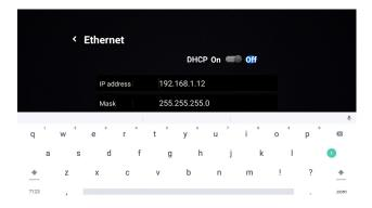
Enter the IP address manually. It is recommended to use a USB keyboard and mouse. Highlight the arrow key on the onscreen keyboard (where the enter key is normally found). Once it is selected, press enter on the keyboard or the OK button on the remote to move to the next line item.
