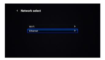
If a DHCP server is on the network, the IP address and associated fields will automatically be filled in. Otherwise the fields must be manually entered.
