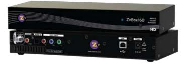
ZvBox® 160 is an HD MPEG-2 Encoder and frequency agile QAM Modulator. It allows you to convert any Component HD video source, in real-time and very high quality into an HDTV cable channel. This channel is placed onto standard COAX wiring, where it can be combined with up to 134 other HDTV channels and distributed over an entire premise.
