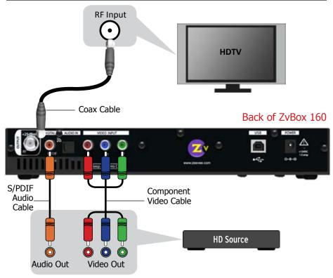
Factory default settings allow your ZvBox to broadcast a component HD source with digital audio on Channel 2.1, over coax cabling, for reception at connected HDTVs.
