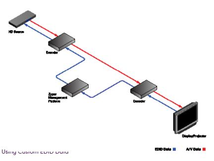
There may be some instances where a custom EDID is desired. One example is when using a single encoder with multiple displays, such as a *video wall*. In such a case, follow the steps below to save and load a custom EDID to the Management Platform.
