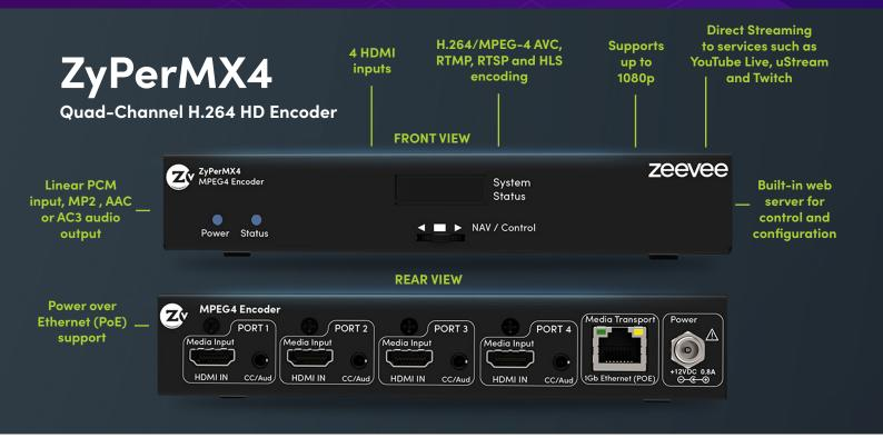
Designed to encode and deliver H.264 video up to 1080p, the ZyPerMX4 allows organizations to deliver content over any IP network. With four encoders in a single appliance, IT/AV managers can deliver more content while utilizing fewer network resources.
