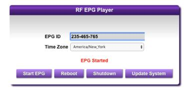
ZeeVee modulator. (ZvPro810 for example). The EPG should be assigned an RF channel so that it can be tuned to just like any other available channel.
