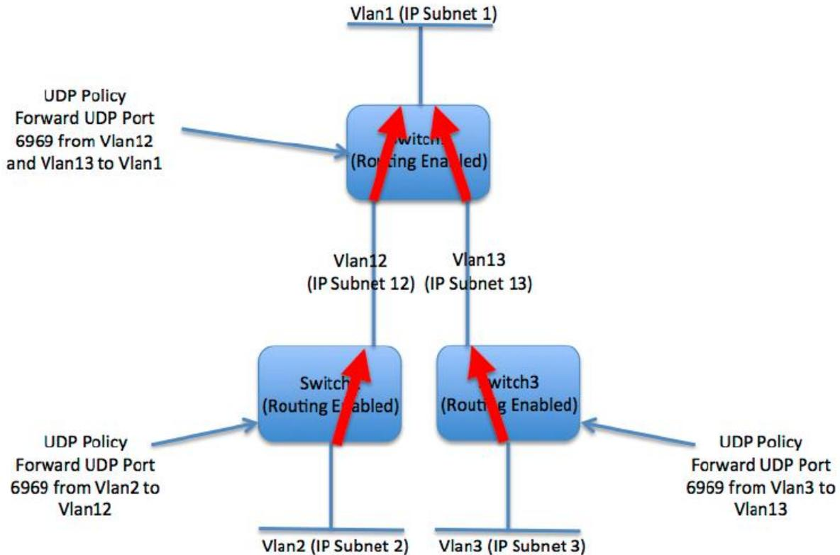
**Special Note:** ZyPer4K endpoints that contain USB need to also have UDP port 6137 forwarded from the ZMP to all endpoint VLANs.
