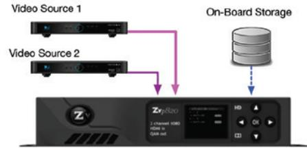
*The user loads a video clip into an internal on-board storage. That video clip is encoded and played just as if it had come from a different video source.*
