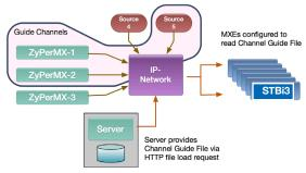
In the diagram shown, if the guide file is specified as exclusive, and the only entries in that guide file are for ZyPerMX-1, ZyPerMX-2, and Source 5, then any other channel will be ignored and not included in the guide. The only stream the user will be able to select are for the channels described in the auide file.
