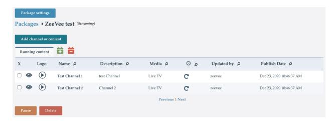
Example above shows the Package "ZeeVee test" with two created streaming channels. To create a new channel, click the "Add channel or content" button.
